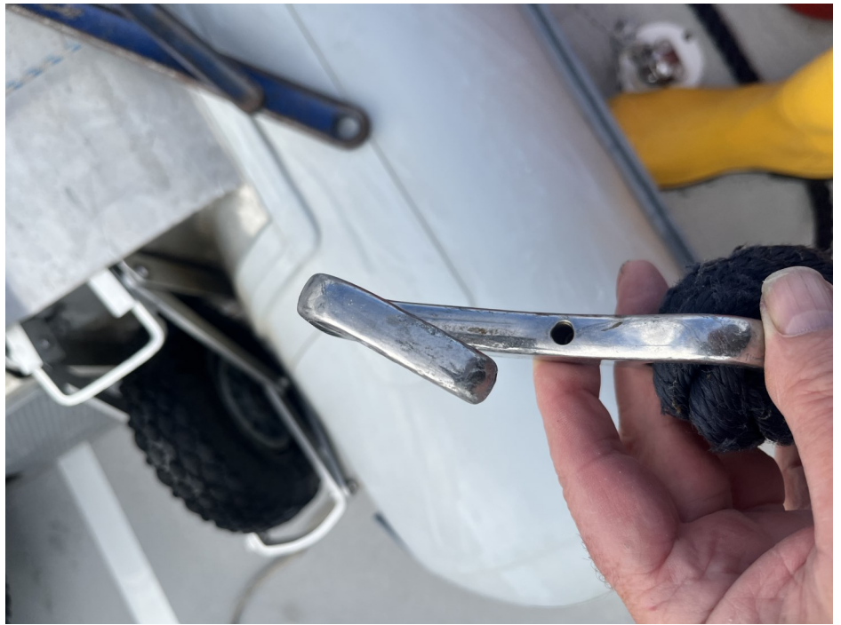
This is the hook from the anchor snubber, it goes through a link on the chain and takes the load on a separate rope—it should be straight but got bent in one of the windy anchorages. With the aid of a vice at the outboard repair shop I was able to straighten it.
