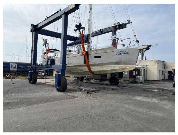
Lifted out at Ardrossan waiting to be pressure washed. The anti fouling paint had done a good job with very little growth on the hull.
